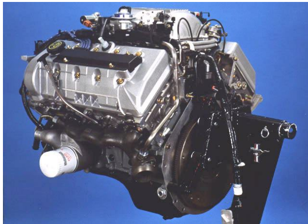
The DOHC Modular V8 in the SVT Mustang is one of the finest V8's ever produced. The physical resemblance to the Boss 429 has to be intentional.
