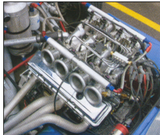
The Beck Lister was the low cost entry. But Beck did fudge a bit, claiming $5,000 for his engine package. Heck, the sexy cross ram fuel injection setup cost more than that. Maybe Beck will give you the rest of the engine for free if you ask him. Car and Driver photo.
