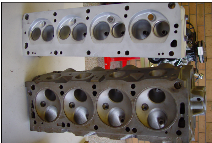
The aluminum over head valve (OHV) medium riser head with inline valves (top), and the hemi single overhead cam (SOHC) head with opposed valves.
