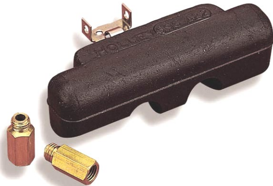
Figure 12: Main Jet Extensions and Notched Float Part 116-10
