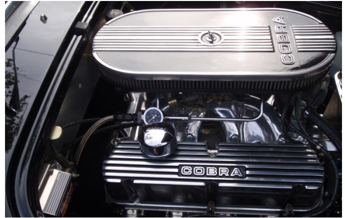
Chuck Juergens SP 840 - rerouted fuel line
