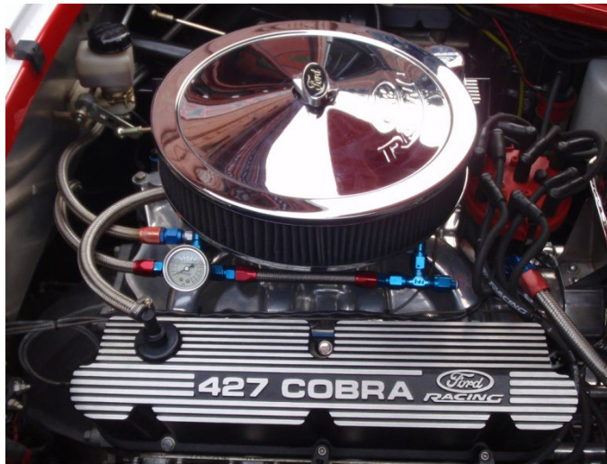
Larry Peet SP 1876- bypass regulator before the fuel log. The regulator is behind the fuel pressure gauge.
