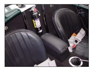
During an extended road-trip in upstate New York, Tony Revetti (SP 1085) realized there was something he needed in his Mk III. He built a custom fit, high quality center console incorporating key features for driver and passenger, as well as providing additional storage for the odds and ends that tended to litter our cars during longer road-trips.
