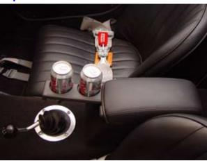
The left tab raises the lid. The right tab slides out to provide a two position cup holder.
