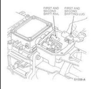
Rotate shifting selector rail moving selector finger away from the thrid and furth shifting lug.
