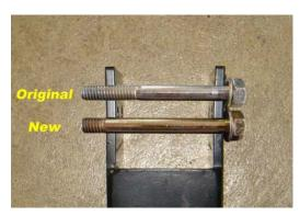
New 8mm, Class 10.9 bolts are available at Advanced Automotive Technologies Corporation 262-673-4077 <a href="http://superformance.org/mountupgrade">http://superformance.org/mountupgrade</a> or you can use 5/16" Grade 8 bolts from suppliers such as <a href="https://www.aircraftspruce.com">www.aircraftspruce.com</a> part number AN5-27A
