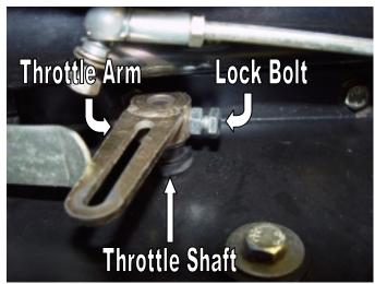
Throttle arm with new lock bolt retainer. View is looking down on assembly from the driver's side.
