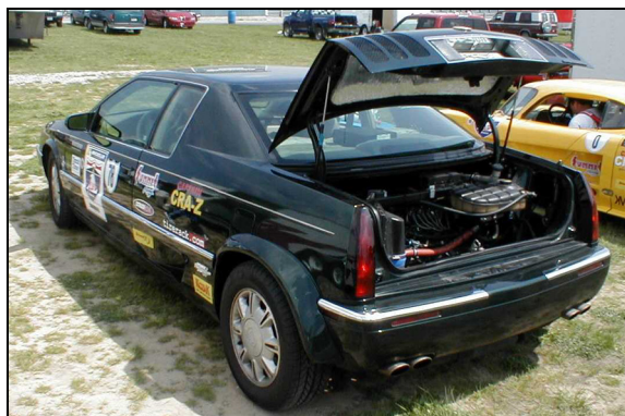
Another Mosler creation. That is a second Northstar V8 in the trunk of the Eldorado.
