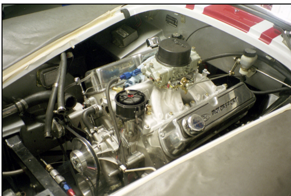
The all aluminum 351W Coupe engine was checked out for 500 miles in SP171, the Olthoff's "test mule".
