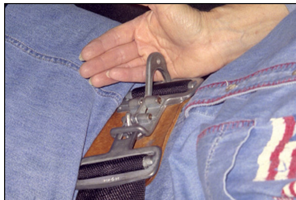
For quick release, swipe the "duck head" as shown.
