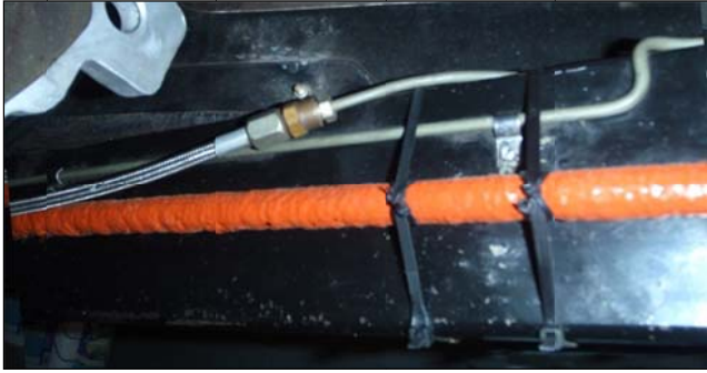
Secure Insulated Steel Fuel Line to Frame with Cable Ties
