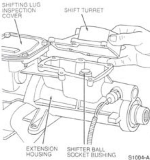
Remove fur shifting lug inspection cover bolts and star washers.
