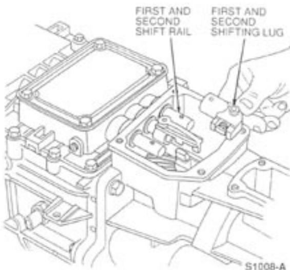
Rotate shifting selector rail moving selector finger away from the third and fourth shifting lug.
