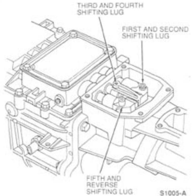
Note: Insert a magnet into area under shifting lugs to catch roll pins when pushed free.
