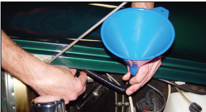
[Figure 53 – Filling Brake Master Cylinder]
