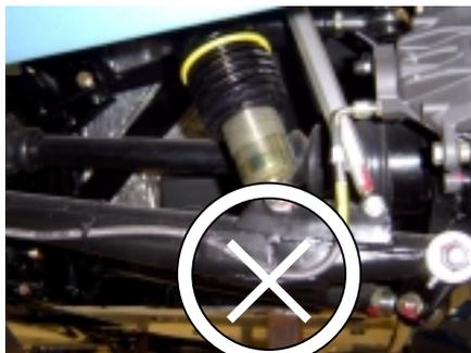
**[Figure 42 - Scissor jack locating point for right hand rear suspension]**
