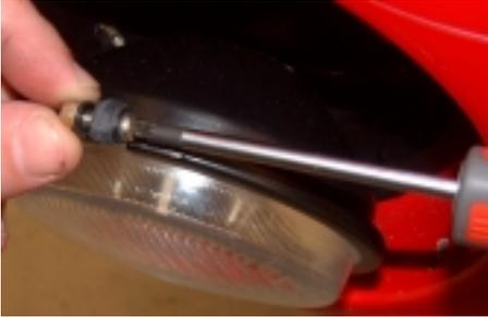
[Figure 67 - Remove fastening ring]
