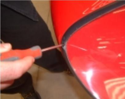
**[Figure 55 - Remove fastening screw]**
