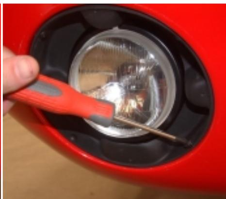
[Figure 66 - Plastic spot light shroud]
