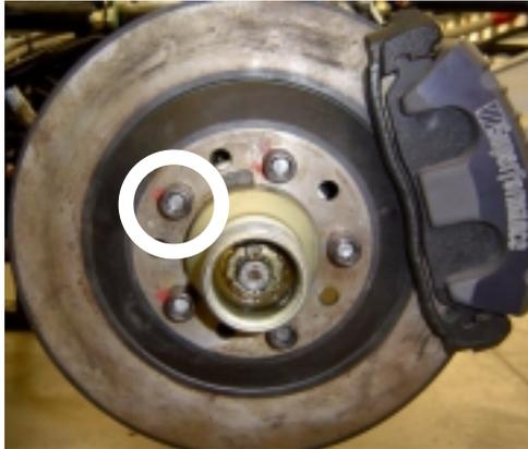
**[Figure 44 – Drive pins on hub center]**
