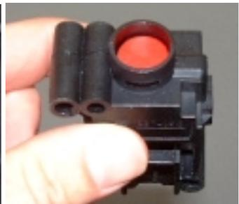
[Figure 19 - Fuel inertia switch]
