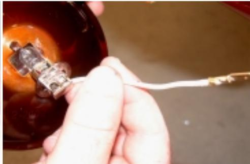
[Figure 70 - Replace bulb and wire]
