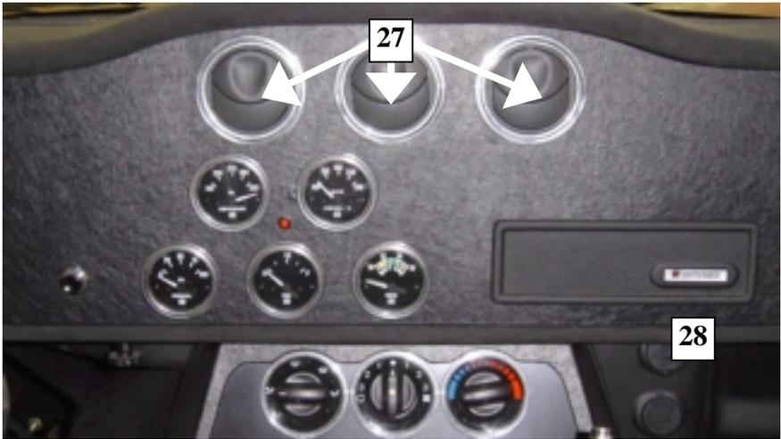
[Figure 10 - Adjustable air vents]
