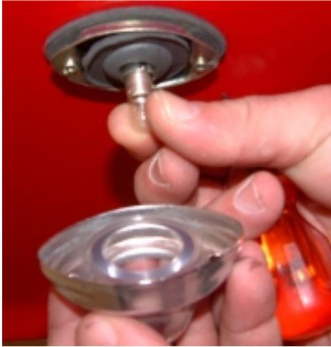
**[Figure 73 - Removal of number plate lamp cover]**
