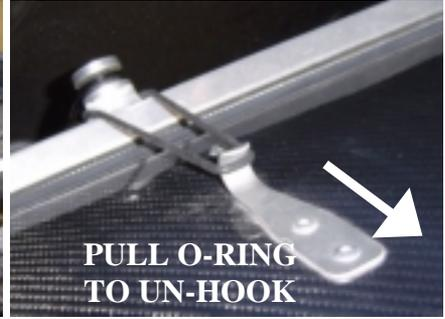
**[Figure 79 - Cowl fastener O-ring]**
