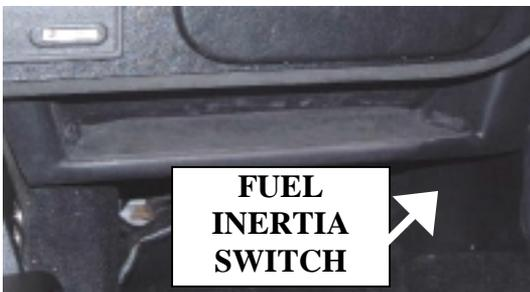
[Figure 18 - Fuel inertia switch location]
