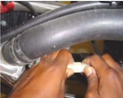
**[Figure 76 - Radiator fan plug - left hand]**
