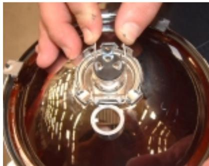
[Figure 64 - Compress spring clip and remove bulb]
