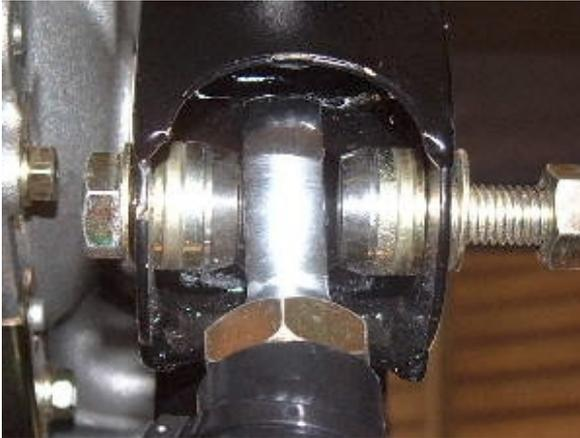
**[Figure 49 – Setting rear static toe]**
