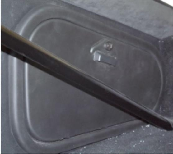
[Figure 26 - Scissor jack compartment]
