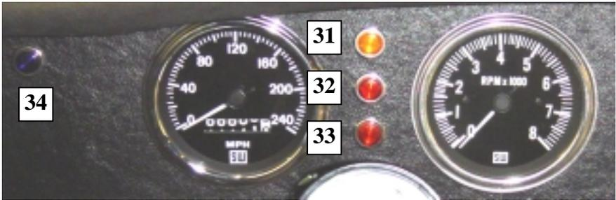
[Figure 17 - Warning lights and buzzers]
