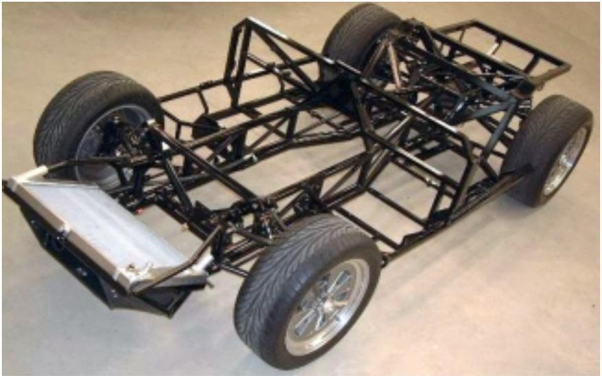
**[Figure 2 – Superformance Chassis, Front View]**
