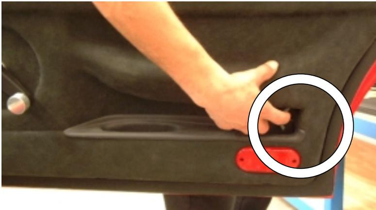
**[Figure 13 - Manual operation door lever]**
