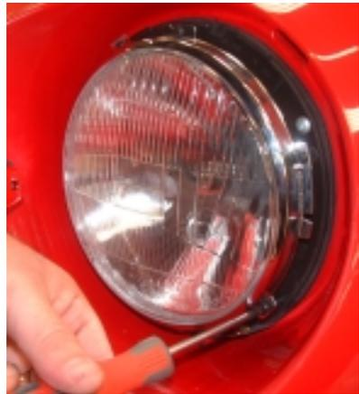
**[Figure 62 - Remove lens fastening screw]**
