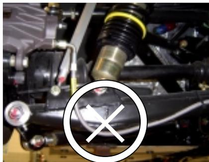
**[Figure 41 - Scissor jack locating point for left hand rear suspension]**
