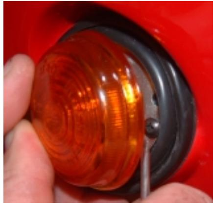
[Figure 72 - Remove indicator lens]
