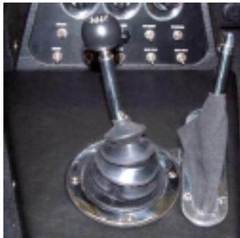
[Figure 15 - Hand brake and gear lever]
