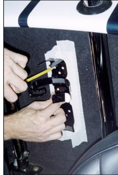
bracket. Only two mounting screws are required, but I elected to use 4 (more is better?). There were three pairs of holes. I elected to use the middle and lower pair. The upper pair is too high and would require drilling into the upper frame crossmember. I aligned the
