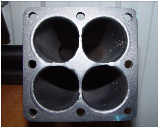
New Superformance exhaust pipe flange showing intact bridge between pipes.
