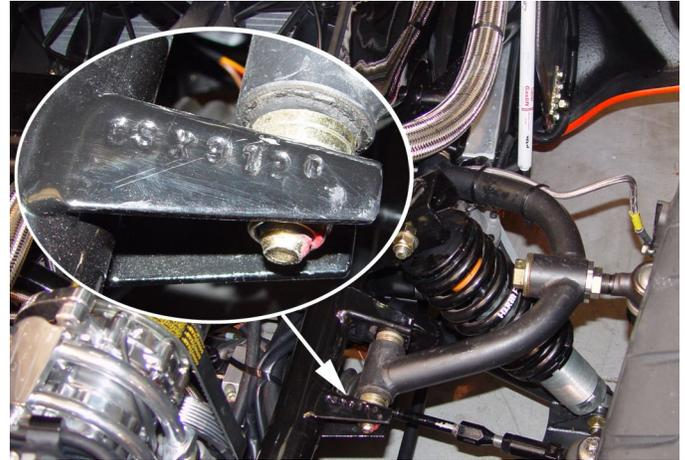
The CSX9000 chassis number is stamped on the rear-most frame mount for the right hand side upper front A-arm.
